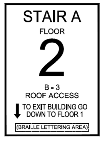
INTERIOR STAIR SIGNAGE EXAMPLE
