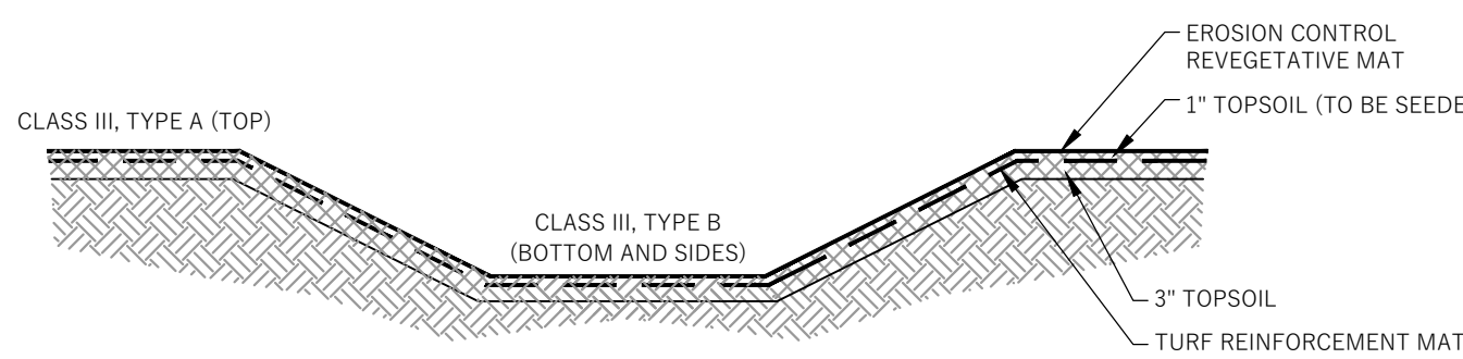
TURF REINFORCEMENT INSTALLATION DETAIL
